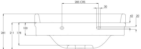
ALL SHOWN DIMENSIONS ARE IN MILLIMETERS AND ARE SUBJECT TO STANDARD CERAMIC TOLERANCES.
