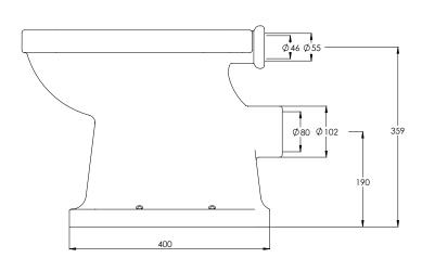
ALL SHOWN DIMENSIONS ARE IN MILLIMETERS AND ARE SUBJECT TO STANDARD CERAMIC TOLERANCES.
