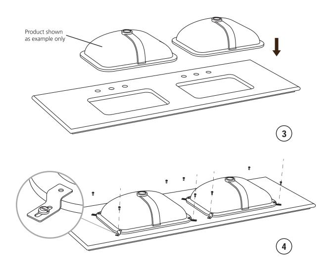
**3** Prepare a clean and protective surface. Carefully place the countertop face down onto the surface.
