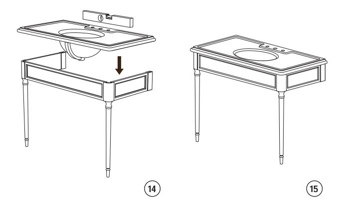
Carefully lower the countertop onto the batten and frame and position in place. Check with spirit level.
