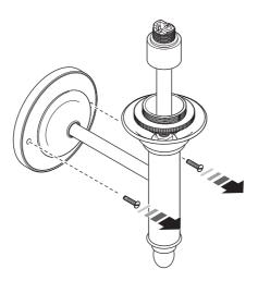
2 Place the mounting plate on to the mounting surface. Mark the location of the upper and lower fixing holes on the mounting surface. Use a spirit level to ensure that the marked locations are vertical. Drill two suitable holes for the required fixings. Wall plugs and screws are supplied with the lamp. Feed the supply cable through the grommet in the mounting plate. Secure the mounting plate using suitable fixings.
