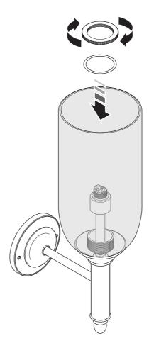
II Gently push the bulb in place before screwing the protective shroud onto the housing.
