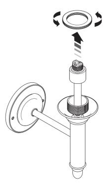
8 Locate the shade onto the lamp body.
