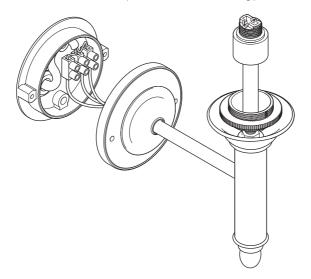
6 Secure the lamp to the mounting plate using the two screws previously removed.
