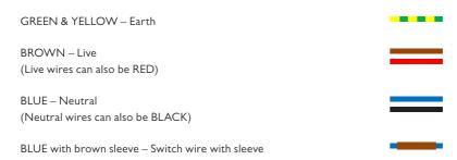
NOTE: Some lamps may have a clear cable. In this case, the earth wire will be marked with a green & yellow thread.
