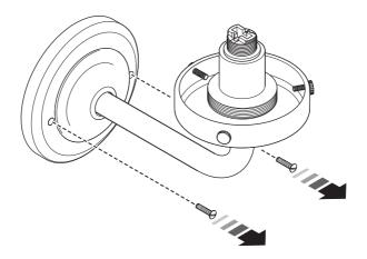
2 Place the mounting plate on to the mounting surface. Mark the location of the upper and lower fixing holes on the mounting surface. Use a spirit level to ensure that the marked locations are vertical. Drill two suitable holes for the required fixings. Wall plugs and screws are supplied with the lamp. Feed the supply cable through the grommet in the mounting plate. Secure the mounting plate using suitable fixings.
