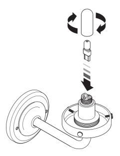
8 Screw the shade in place to cover the bulb. There is no need to tighten the shade, gently rotate it until it stops.
