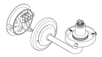
6 Secure the lamp to the mounting plate using the two screws previously removed.
