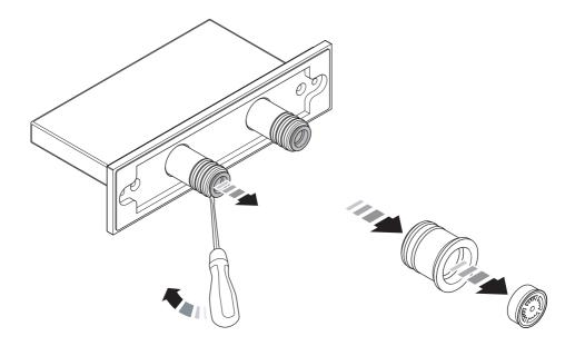
5 There are flow regulators located in the rear of the spout connectors. For cleaning purposes, insert a flat blade screwdriver behind the raised lip of the regulator housings to remove. The regulators can be pushed from the housings using a finger, never use anything sharp as this may damage the regulator. Simply push from inside the housing as shown above.
