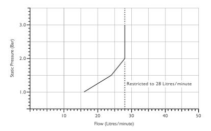
Note: Balanced pressures shown are applied directly to the hot and cold inlets; flow rates indicated are free flowing and may vary subject to restrictions created by installation, pipework, layout or application.
