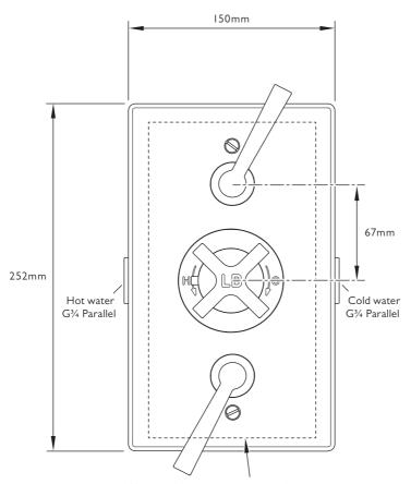
230mm x 120mm aperture behind face plate for maintenance access
