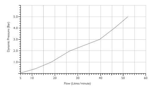
Note: Balanced pressures shown are applied directly to the hot and cold inlets; flow rates indicated are free flowing and may vary subject to restrictions created by installation, pipework, layout or application. Upper and lower outlets have the same flow rates.
