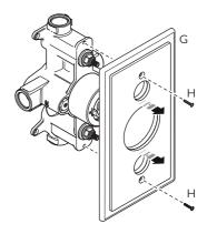
4 To remove the facing plate (G) unscrew and remove fully the 2 fixing screws (H). Carefully prise the facing plate off the wall using a flat bladed screw driver (the gasket is reusable).
