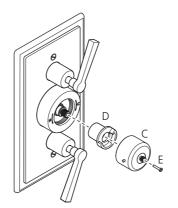
Remove the override (C) and temperature stop (D) by unscrewing and removing screw (E).
