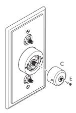
3 Remove the override (C) by unscrewing and removing screw (E).
