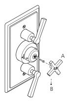
Remove the thermostatic control cross handle/ handwheel (A) by unscrewing set screw (B) using a 1.5mm hexagonal key.
