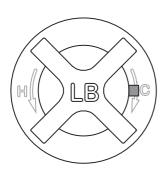
Safe temperature button set to right (suitable for left handed operation)
