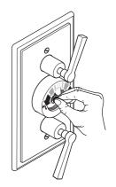
Adjust the cartridge spline whilst measuring the temperature of the water. Ideally the temperature measurement should be taken using a digital thermometer.
