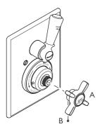
Remove the thermostatic control cross handle (A) by unscrewing set screw (B) using a 1.5mm hexagonal key.
