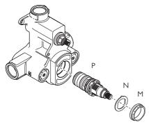
7 To remove the thermostatic cartridge, unscrew and remove locking nut (M). Remove anti-rotation washer (N) and pull out cartridge (P). To help with cartridge removal, it is recommended you fit override (C) with screw (E) to make pulling the cartridge out easier.
