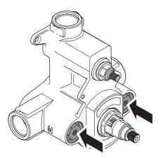
6 Isolate the hot and cold water supplies as follows: The non-return valve covers have a screw in the centre. Use a screwdriver to turn the screws in a clockwise direction until they reach their stop. Do not over tighten the screws as this may damage the non-return valves.
