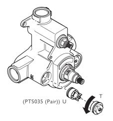
I Isolate the hot and cold water supplies before the shower valve. With the lever, cross handle, override, temperature stop and cartridge cover removed, you can see the non-return valve cover(s). Using a 17mm spanner or socket, unscrew and remove the non-return valve cover(s) (T).
