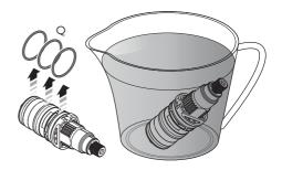
8 Check the 'O' rings (Q) for damage (ie. cuts or tears). A set of three replacement 'O' rings are available (PTS027). Remove the 'O' rings before soaking the cartridge in descaling fluid. Soak the cartridge according to the instructions on the descaling fluid packaging. Rinse under cold water before fitting (refer to the 'installing the thermostatic cartridge' section to install).
