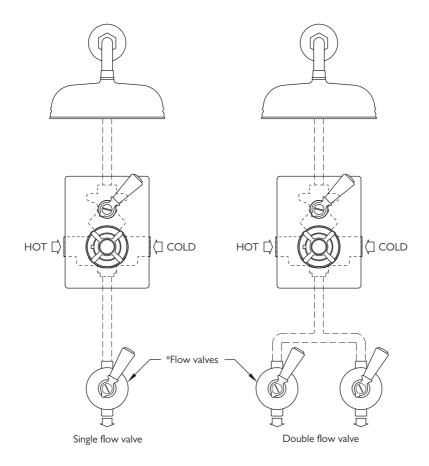
For adding a hand shower, body jets or bath filler, remove the ¾" BSP plug from the bottom of the valve body and connect suitable flow valve(s). \*Flow valves are available as 'DL' (Fifth lever), 'DH' (Fifth cross handle), 'WL' (White lever) & 'BL' (Black lever). (Refer to flow valve installation instructions)
