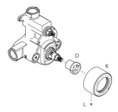
5 Remove the thermostatic cartridge cover (K) by unscrewing set screw (L) using a 1.5mm hexagonal key. Temperature stop (D) can be pulled off.
