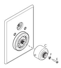
3 Remove the override (C) by unscrewing and removing screw (E) and washer (F).
