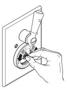
Remove the override (C) and temperature stop (D) by unscrewing and removing screw (E) and washer (F). Fitting cross handle (A) and set screw (B) will aid with removal of override (C). Adjust the cartridge spline whilst measuring the temperature of the water. Ideally the temperature measurement should be taken using a digital thermometer.
