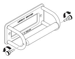
I The paper holder bar is held in place with two thumb screws. Support the bar and unscrew the thumbscrews. Lift the bar clear of the support arms.
