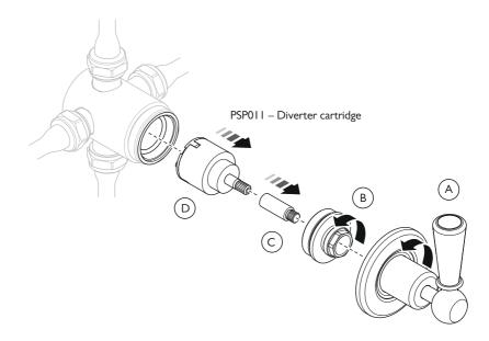
**Problem solving** – Servicing should only be necessary if the diverter fails to divert water, or water is present at two applications at the same time.
